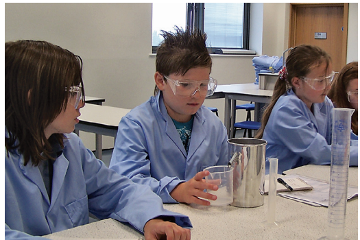
Figure 8 Using a displacement vessel to determine the volume of a piece of limestone in the CELS science laboratories
