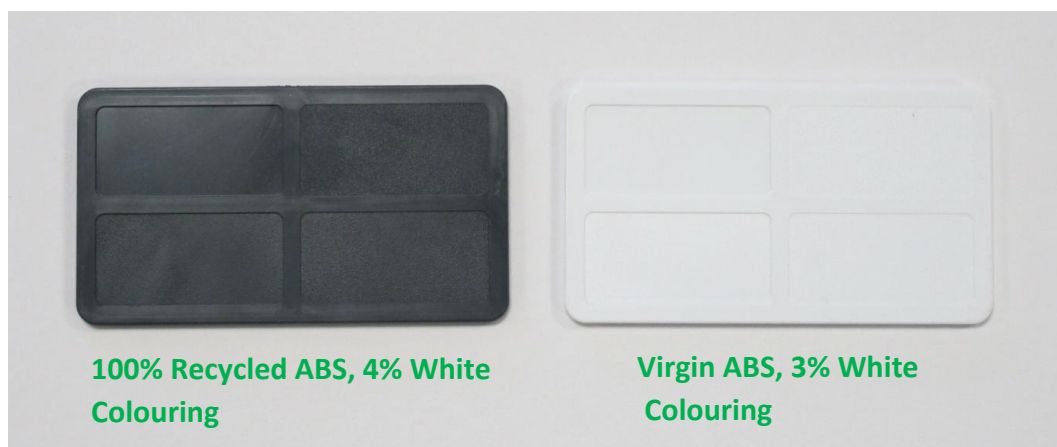
Adding white master batch to test plaques
