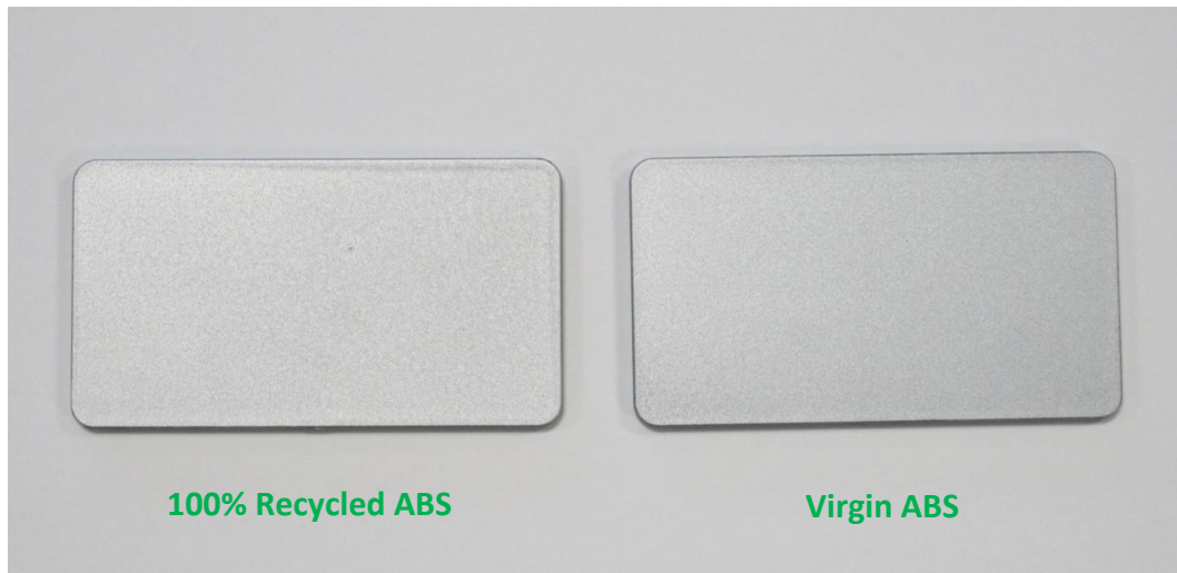
Cellulose based, silver spray paint applied to both materials
