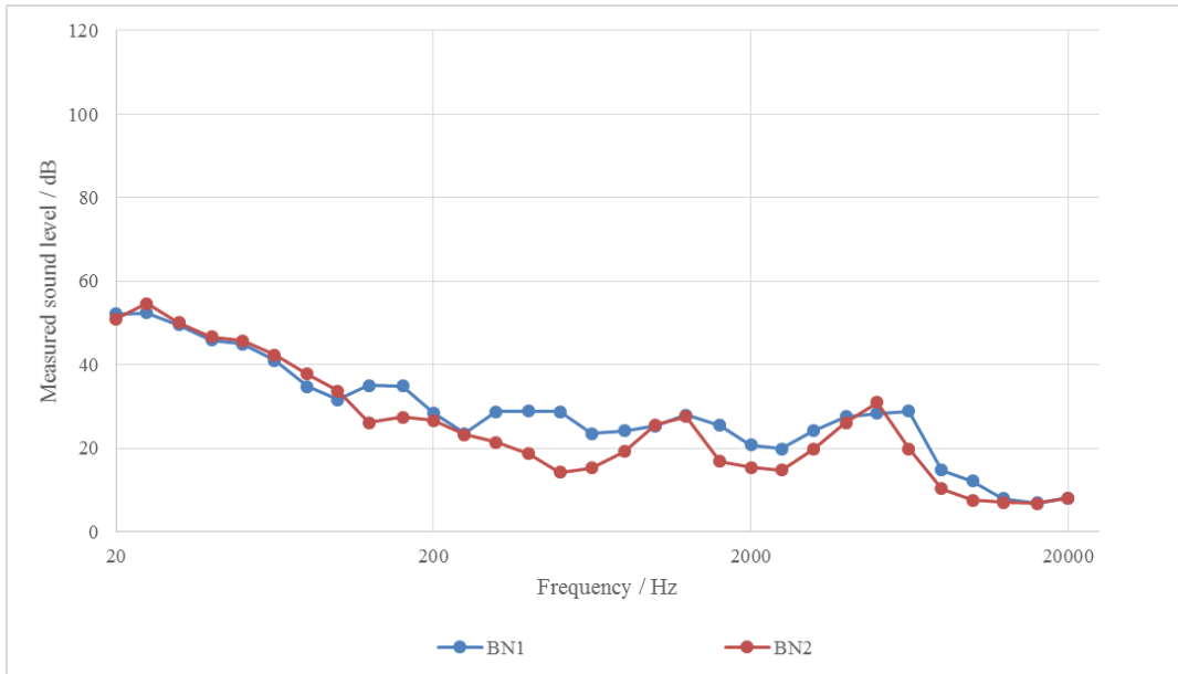
Figure 10. Measured background noise level of the testing environment against the frequency response of the sine sweeping audio input in the frequency range of 20 to 20 kHz in log scale.
