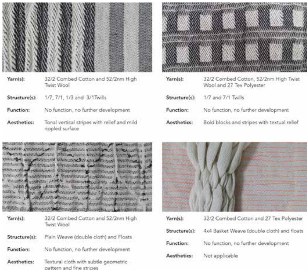
Figure 7.11: Jacquard Technical Samples: Warp and Weft-facing Pleats and 3D Folds (2015) Photographs by Anna Piper
