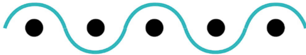
Biaxial Weaving: 1 x warp, 1 x weft
