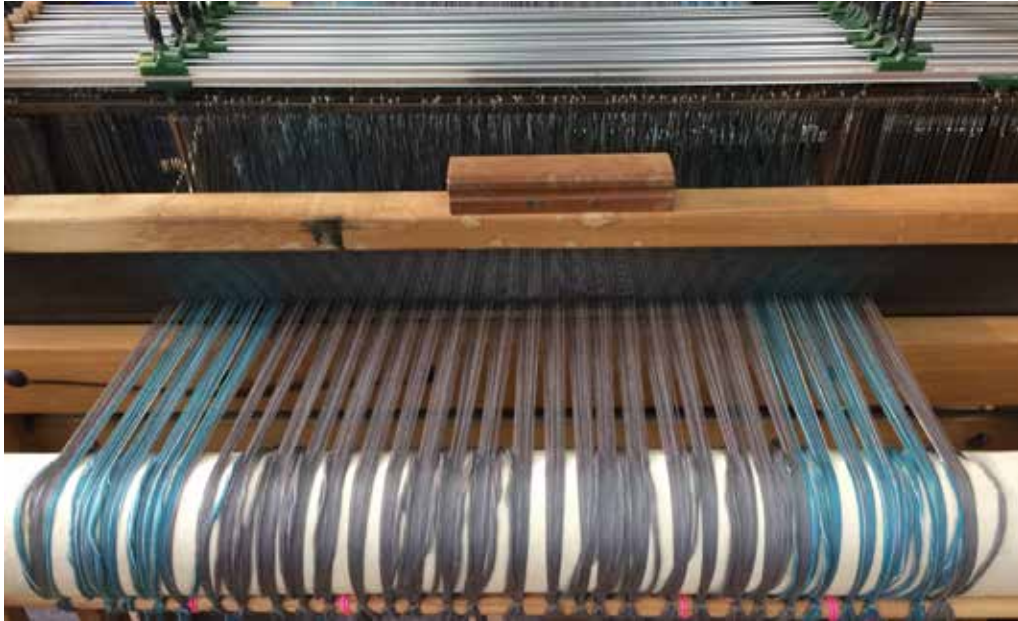
Figure 4.13: The Reed Determining the Width and Density of the Warp (2017) Photograph by Anna Piper
