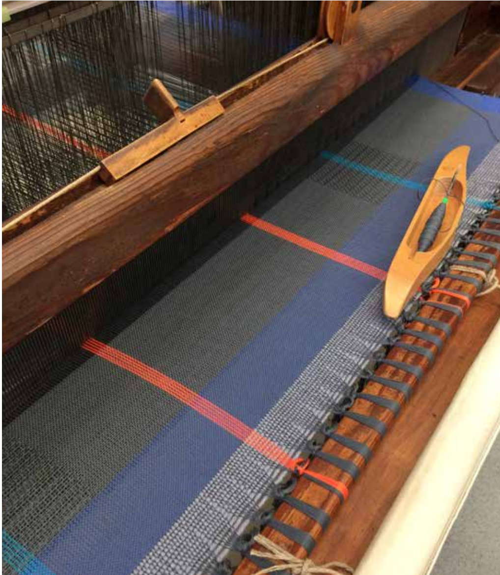
Figure 4.15: Block Threading Facilitating the Panelling of Weave Structures (2018) Photograph by Anna Piper
