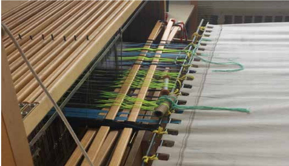
Figure 5.7: Unusable Warp Threaded Through Heddles (2018) Photograph by Anna Piper
