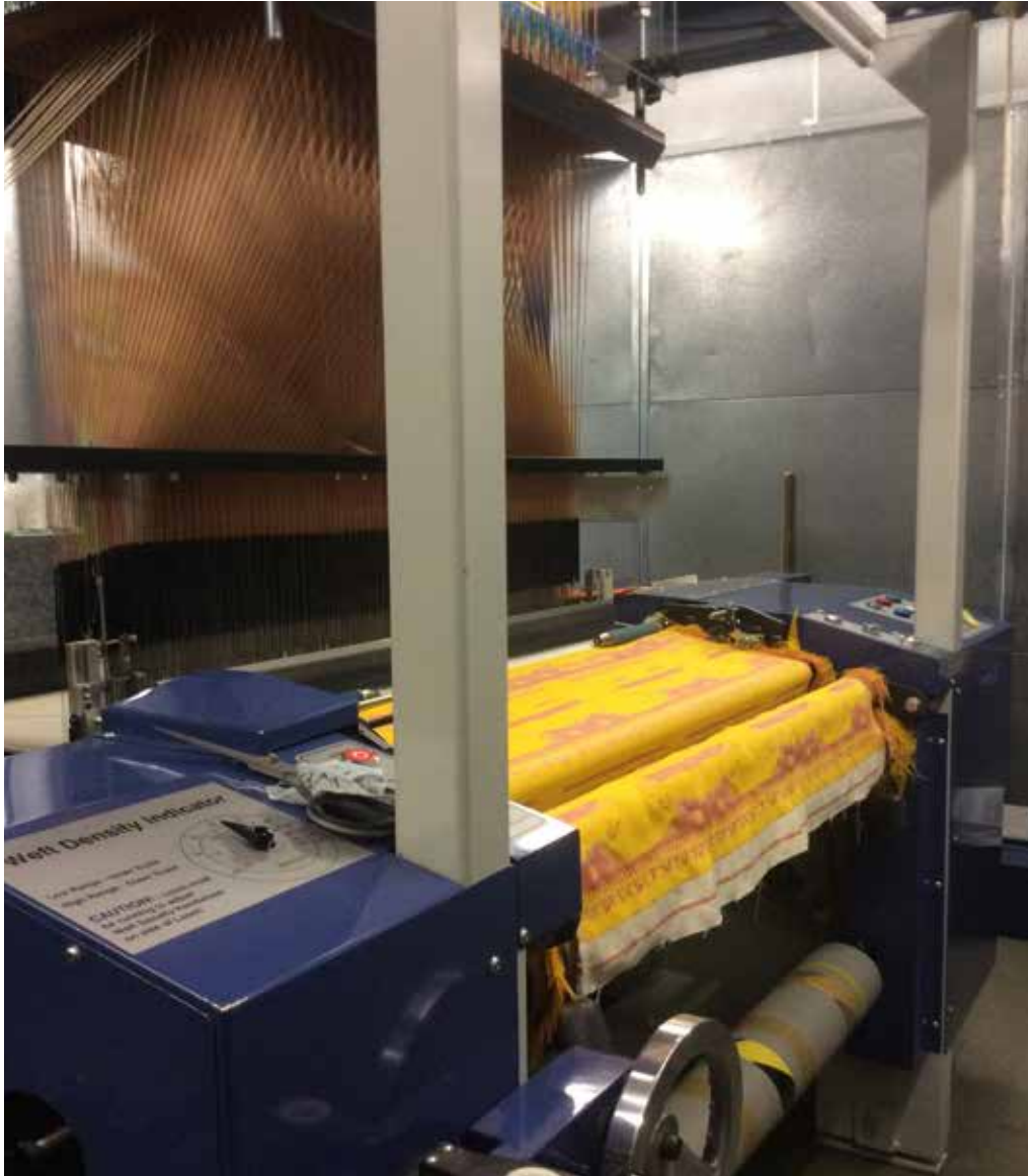
Figure 7.3: Bonas Sample Master Digital Jacquard Power Loom (2018) Photograph by Anna Piper
