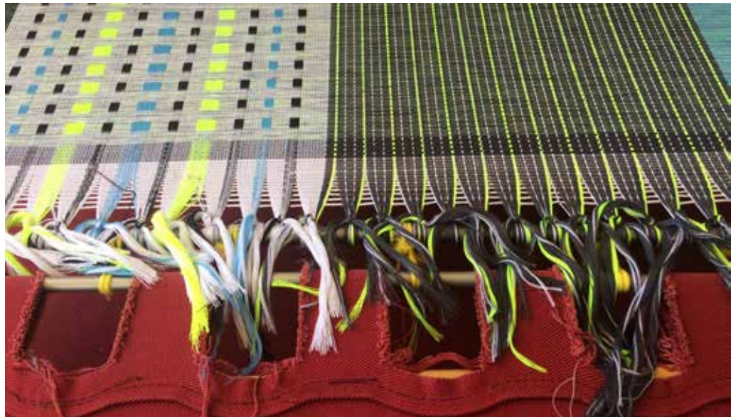
Figure 5.8: Warp Tied to the Front Beam (2018) Photograph by Anna Piper
