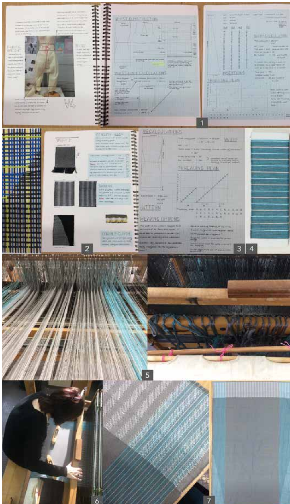
Figure 7.16: Hand Woven Trouser Production Process (2017) Photographs by Anna Piper
