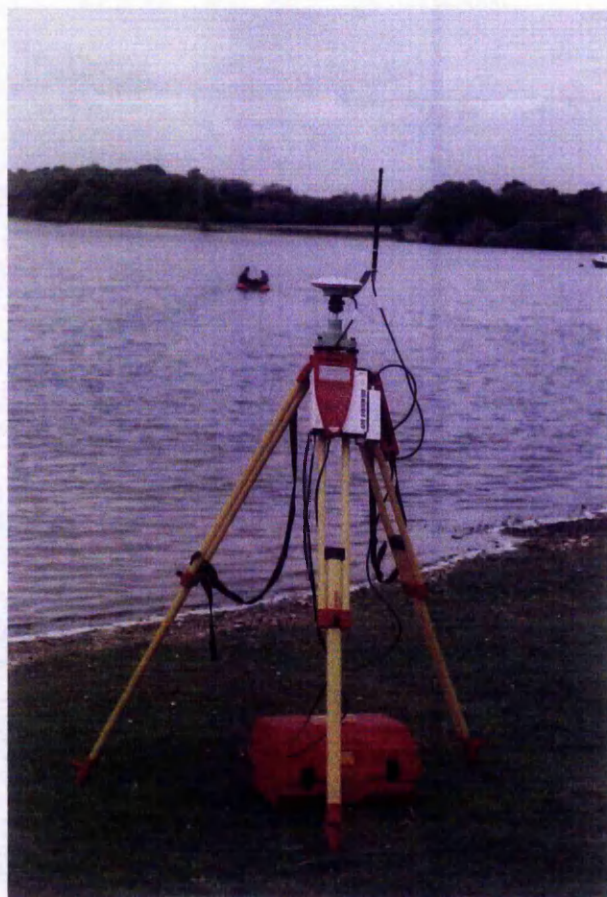
Figure 4.7 Bathymetric survey - differential GPS
