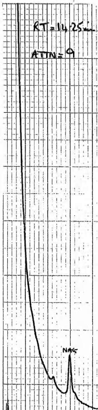
Figure 21. 0.1 g/L of N-acetyl glucosamine reacted with TRISIL. Column: 2 metre OV11. G.L.C. conditions: oven 200°C, carrier gas nitrogen 20 mL/min, Flame Ionisation Detector 225°C, injector 250°C.
