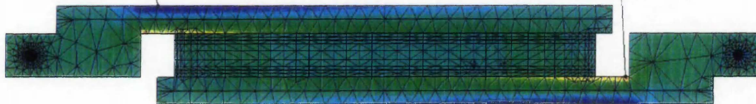
Figure B5.5a BS 4370 worst principal stress contour plot and mesh density
