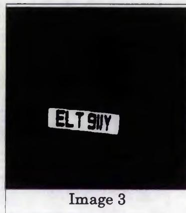
The outline of the plate is only important in that it helps to determine if the plate region has been correctly identified. In all images except image 5 the outline of the plate is complete. However, even Image 5 has a substantial amount of the plate visible, adequate to confirm that it is a plate. A more important aspect of the images is the clarity of the characters. Ideally each character should not be touching either its neighbours or the black background of the image.
