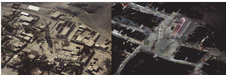
Figure 2 (left) Poirot, F. Aerial view of Tarapacá in 1978-1979. Source: http://www.panoramio.com/photo/1536741 / Figure 3 (right): Same view as before but obtained using the 3D point cloud from the scans taken in 2013. Source: B. Devilat
