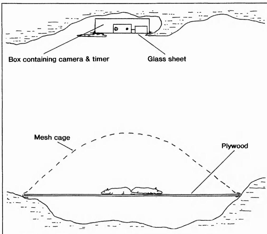
Figure 2.4: Apparatus to monitor post-mortal movement *in situ* (not to scale).
