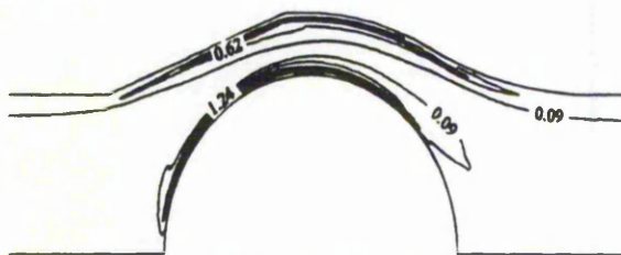
Figure 8: Shear stress contours for Re=500
