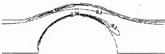
Figure 3: Shear stress distribution (Q=2.97l/m, H=21%).
