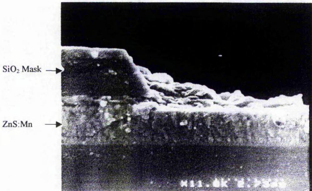
**Figure 5.4** SiO<sub>2</sub> mask on ZnS:Mn thin film before ion milling
