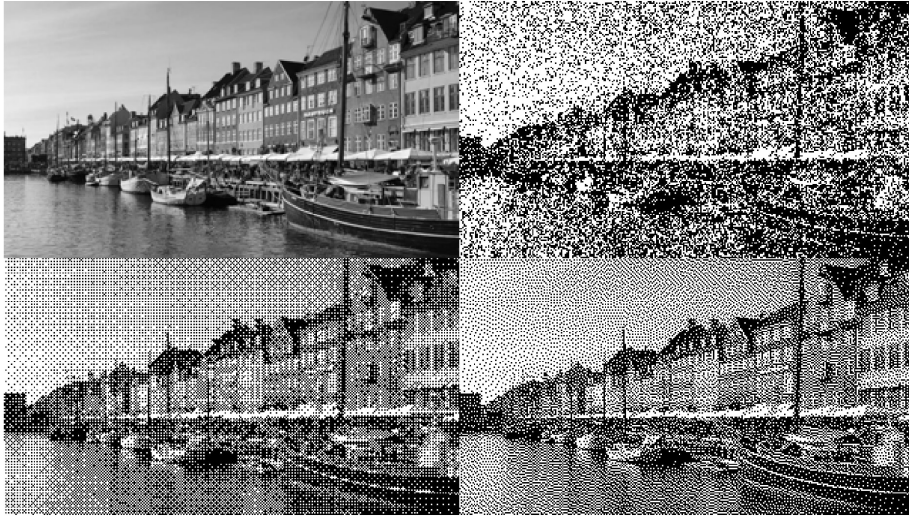
Figure 1: Image showing the different 2D dithering algorithms. Top Left = Original Image, Top Right = Random dithering, Bottom Left = Bayer dithering, Bottom Right = Error Diffusion dithering.
