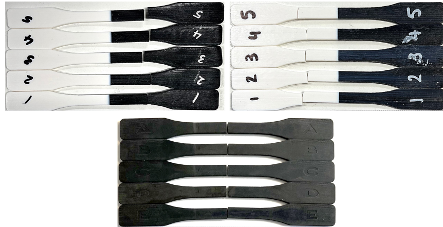
Figure 16: Failure locations within PI parts of all material combinations. Left = VW/AB, Centre = VW/VB, Right = ABS/ABS.
