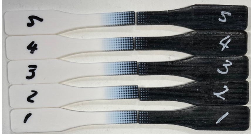
Figure 12: Failure Locations for the VW/AB SP 20 mm samples.
