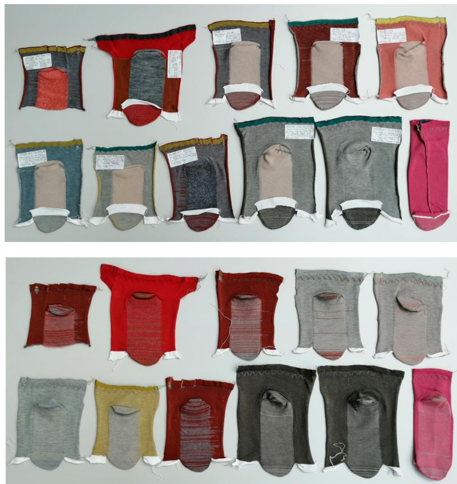
Figure 6-2: Sampling with different yarn qualities to resolve the plush and plating technique. See Appendix 10. for detailed yarn combinations (Lisa Shawgi, 2018).
