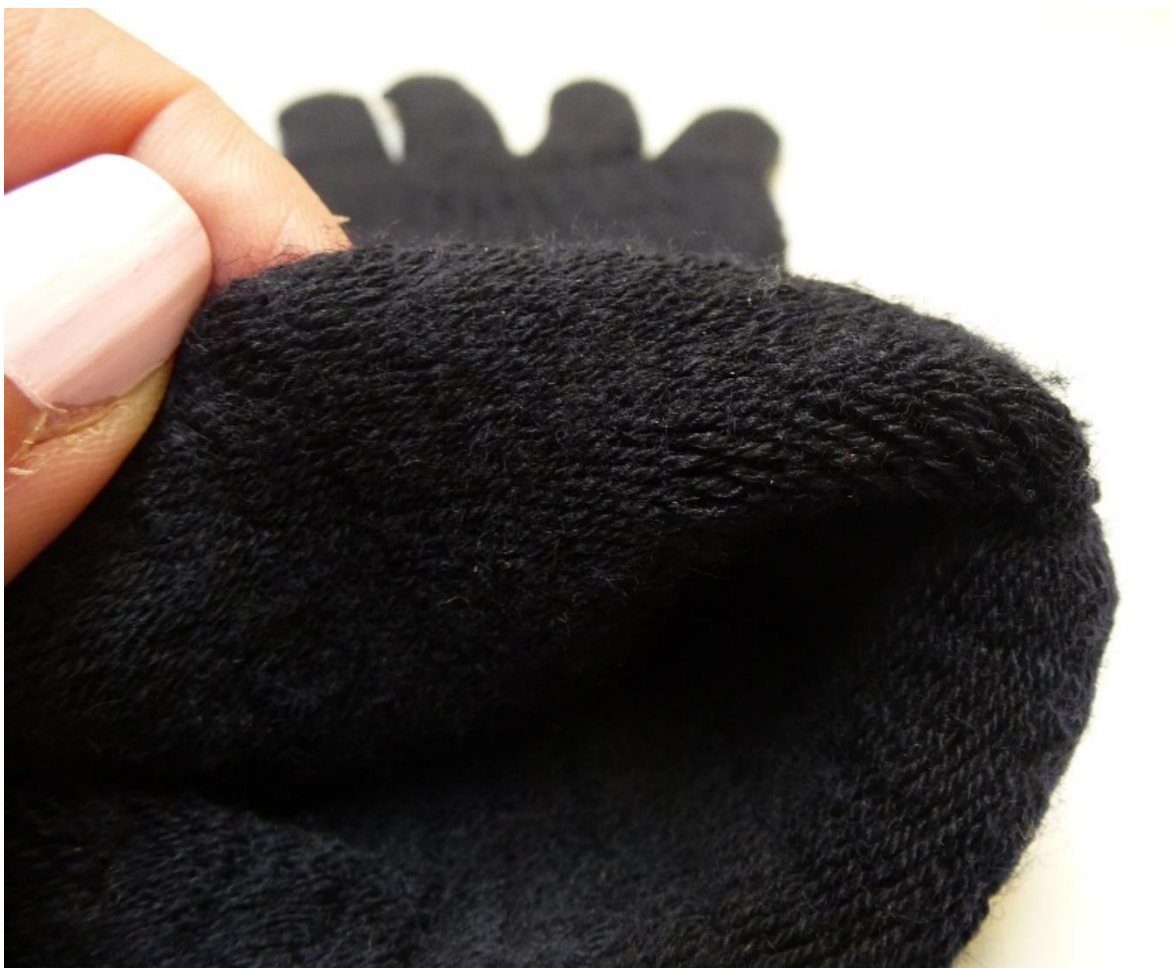
Figure 8-19: Inside of glove showing the ‘floating tuck’ technique (Lisa Shawgi, 2019).
