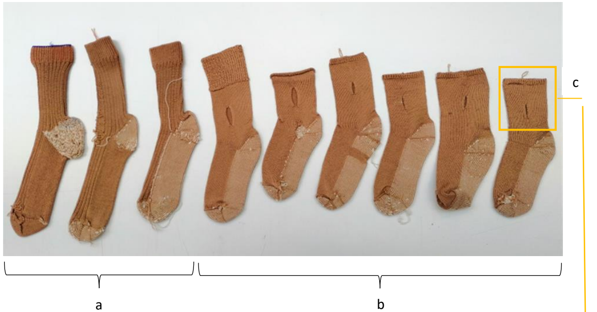
Figure 7-3: From left to right, development of sock prototype using Stoll, CMS ADF 32W, Multi gauge machine (Lisa Shawgi, 2018).
