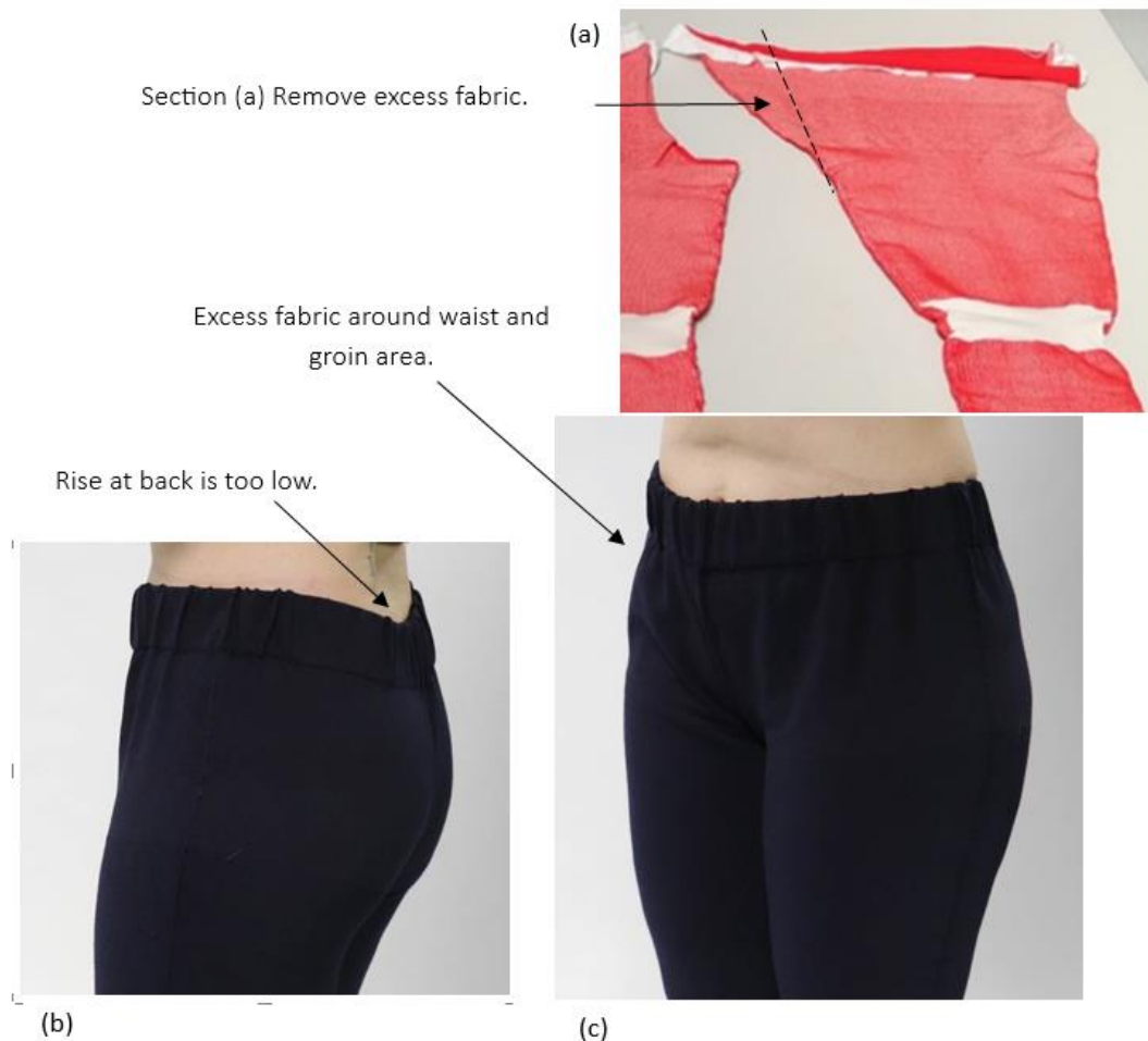
Figure 8-15: Image (a): detail showing the need for the removal of more fabric alongside the seam of hip and waist areas; Image (b): detail showing rise of leggings; Image (c): detail image showing excess fabric which needed removing (Lisa Shawgi, 2023).
