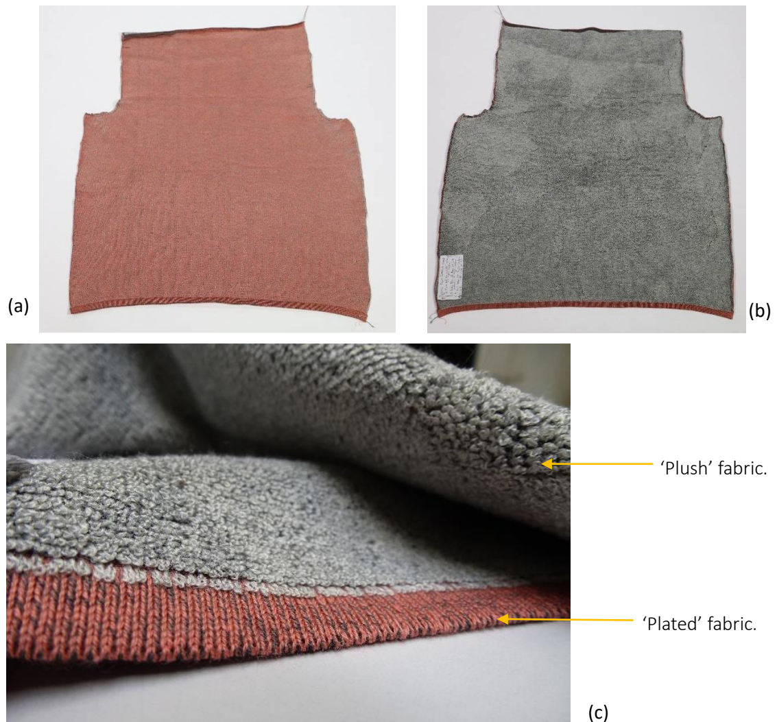
Figure 7-25: Image (a): knit side of back panel; Image (b): purl side of fabric showing the 'plush'; Image (c) is a close up of the 'plush' fabric and some of the 'plated' fabric on the hemline (Lisa Shawgi, 2019).
