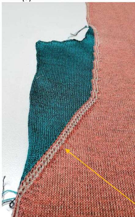
Figure 7-30: Image (a): knit side of front panel; Image (b): purl side of front panel; Image (c): detail showing opening created by tubular knitting to house magnets (Lisa Shawgi, 2019).
