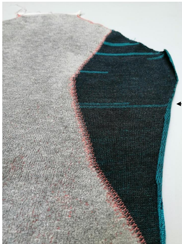
Figure 7-33: Close up of joining and 'plating' issues (Lisa Shawgi, 2019).
