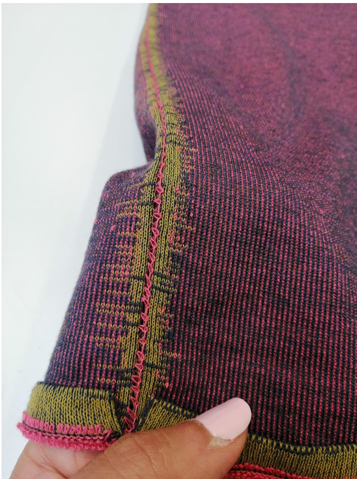
Figure 8-39: Close up of the side seam where both side seams were placed onto the needles and cast off (Lisa Shawgi, 2020).
