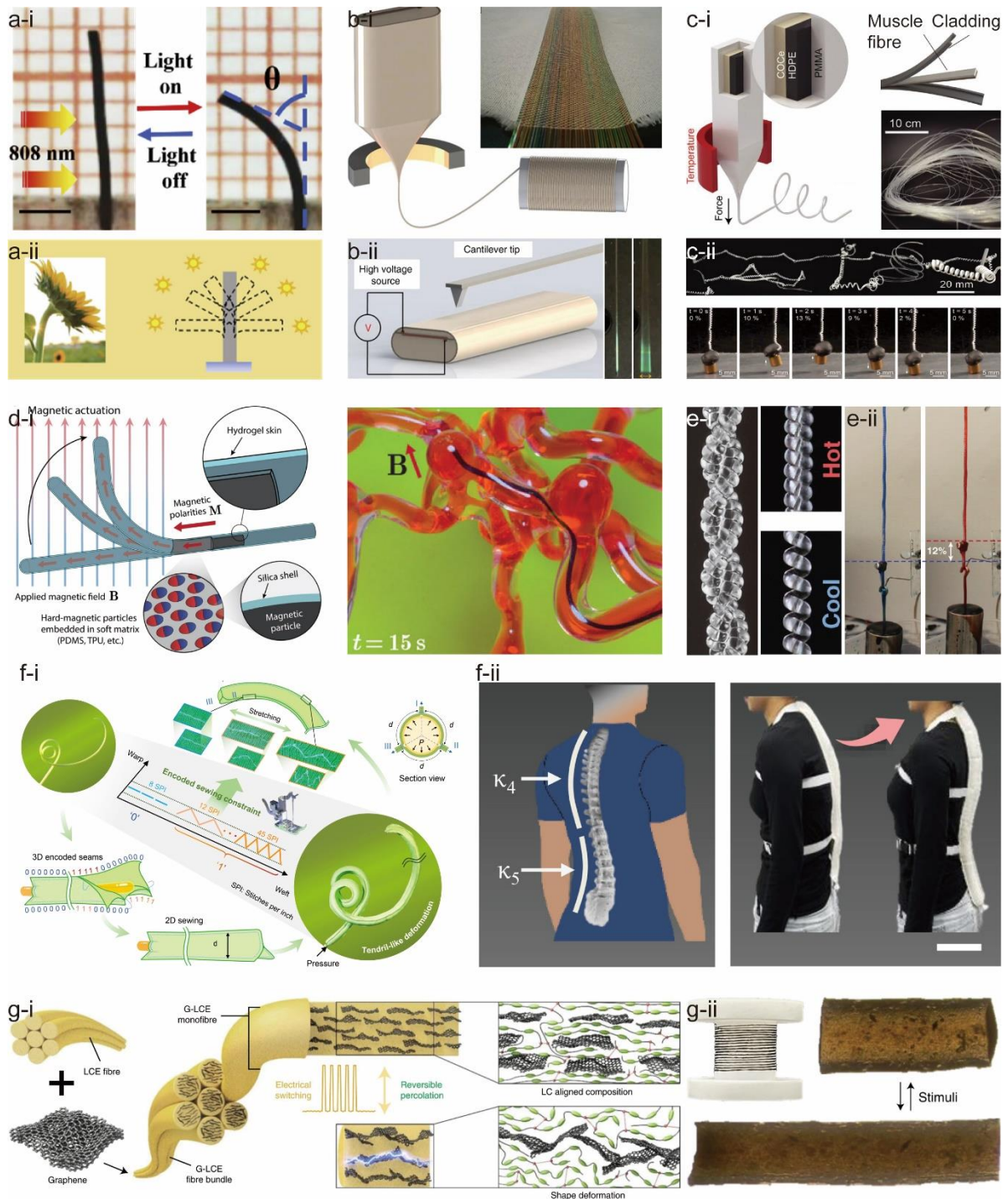
Fig 16. Feedback and actuation: (a-i) Photos of the bending actuation caused by left-side illumination. (a-ii) Photo of the phototropic movement of a sunflower, stimulated by infrared light spots from various incident directions. (a) Reproduced from ref. 352 with permission from Elsevier Ltd, copyright 2022. (b-i) Schematic of the preform-to-fibre draw process (left); An array of flexible electro-strictive fibres exhibiting colored reflections through the Bragg effect (right). (b-ii) The amplitude of oscillation is displayed for both on-resonance and off-resonance frequency points. (b) Reproduced from ref. 353 with permission from Springer Nature, copyright 2017. (c-i) Bimorph fibres produced via two-step thermal drawing. (c-ii) Photographs of the artificial fibre muscles and of them lifting 1 g mass. (c) Reproduced from ref. 260 with permission from American Association for the Advancement of Science, copyright 2019. (d-i)
