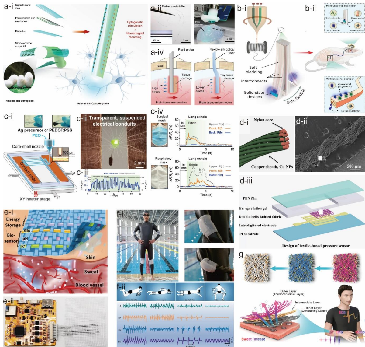
Fig 12. Physiological sensing. (a) A silk-based fibre for neural recording. (a-i) The fibre is prepared with silk protein and integrated with multiple electronic components. (a-ii, iii) The flexibility of the neural fibre allows recording in freely behaving animals. (a-iv) The neural fibre actively adapts to the brain after implantation by reducing its own mechanical stiffness with high fidelity. (a) Reproduced from ref. 325 with permission from Springer Nature, copyright 2022. (b) A thermally drawn fibre probe with multiple solid-state devices for the modulation of neural circuits. (b-i) Fabrication and (b-ii) functions of the fibre probe. (b) Reproduced from ref. 326 with permission from Springer Nature, copyright 2023. (c) Functional mask for breath monitoring via inflight fibre printing. (c-i) The printing process and (c-ii) the printed fibre mesh. (c-iii, iv) Commercial masks integrated with printed fibres are used to monitor breath. (c) Reproduced from ref. 327 with permission from American Association for the Advancement of Science, copyright 2020. (d) Pulse monitoring by fabric sensors. (d-i) Schematic illustration of the fabric made by the fibre with a core-sheath structure. (d-ii) SEM images showing the surface morphology of the fibre. (d-iii) The design of sandwiched textile-based pressure sensor. (d) Reproduced from ref. 328 with permission from Wiley-VCH, copyright 2022. (e) A fabric integrated with reduced graphene oxide/tetra-aniline fibre for continuous monitoring of human sweat. (e-i) The fabric sensor works as a patch attaching to
