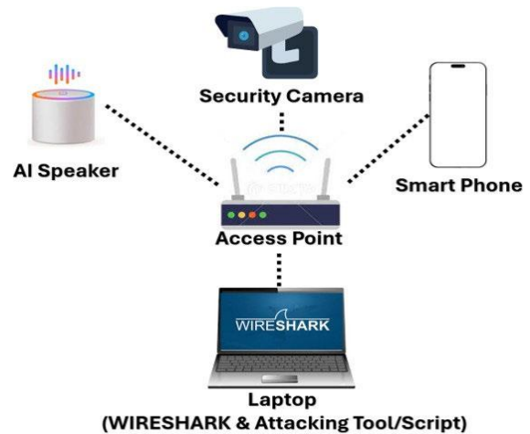
FIGURE 3. IOTID20 dataset testbed environment.
