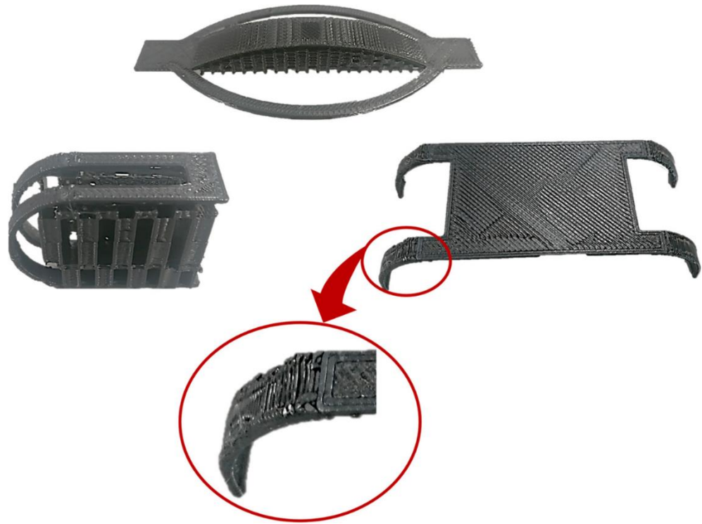
Figure 4.8. Permanent form structures printed in three dimensions with support.
