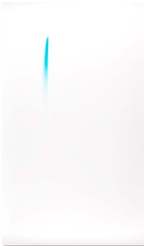
Fig. 26: Fogged paper artefact generated by Chromira's sensor.
