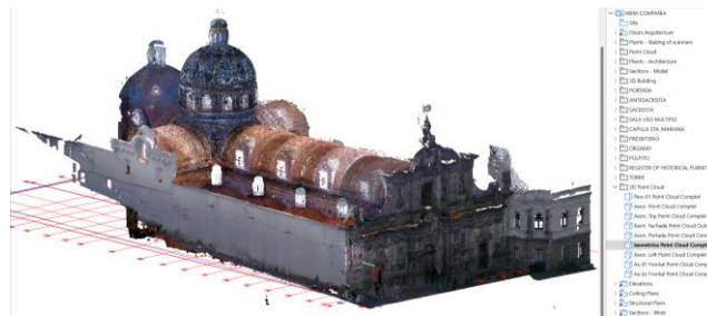
Fig. 2. Global point cloud in the ArchiCAD HBIM project. Isometric view.
