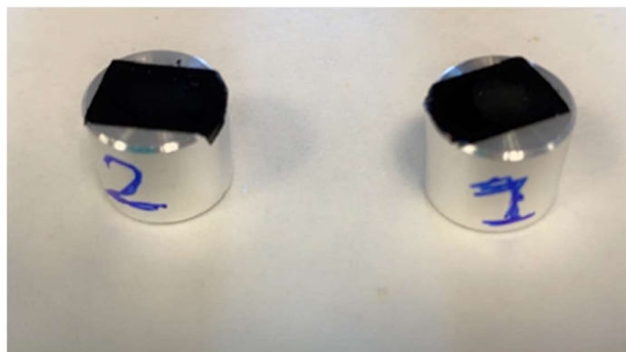
Figure 3.1: Carbon coating for SEM analysis, (sample 1) is the quaternary of perovskite samples \text{Bi}_2\text{Mn}_{1.3}\text{Ni}_{0.7}\text{O}_6 before heating, and (sample 2) after heating.
