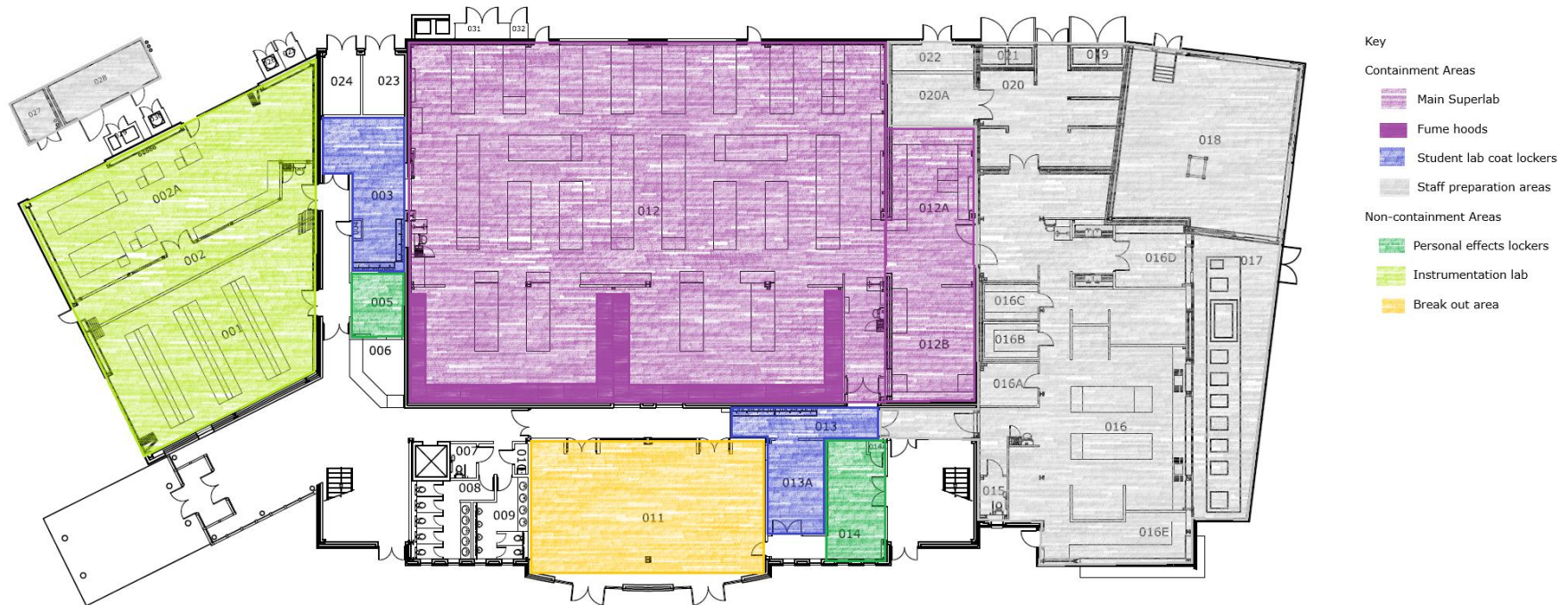
Figure 3: The Rosalind Franklin building ground floor plan, showing the Superlab in purple, decontamination areas and lab coat lockers in blue, and personal locker spaces in green.
