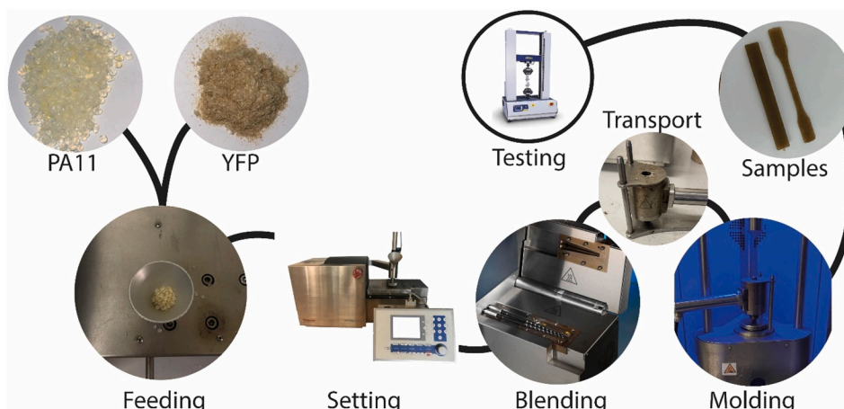
Fig. 2. Fabrication route of injection-molded PA11/Yucca composite specimens.
