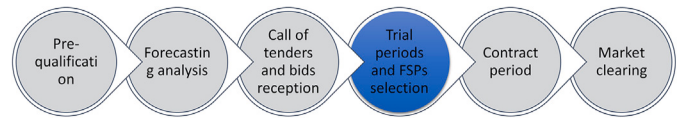
Fig. 2. The timeline of the procedure for contracted flexibility: The DSO launches a call for flexibility (step 3) if a congestion is predicted (step 2). After receiving the offers (step 3), the DSO decides the winning offers (step 4) and signs contracts with the selected providers (step 4). The paper addresses the challenges of step 4, which aims at selecting flexibility providers with the best reliability and lowest costs.
