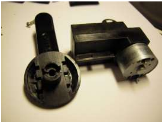
Figure 4.14 Energy system (Crank Handle, Motor, Rechargeable Battery) disassembled from radio (left)
