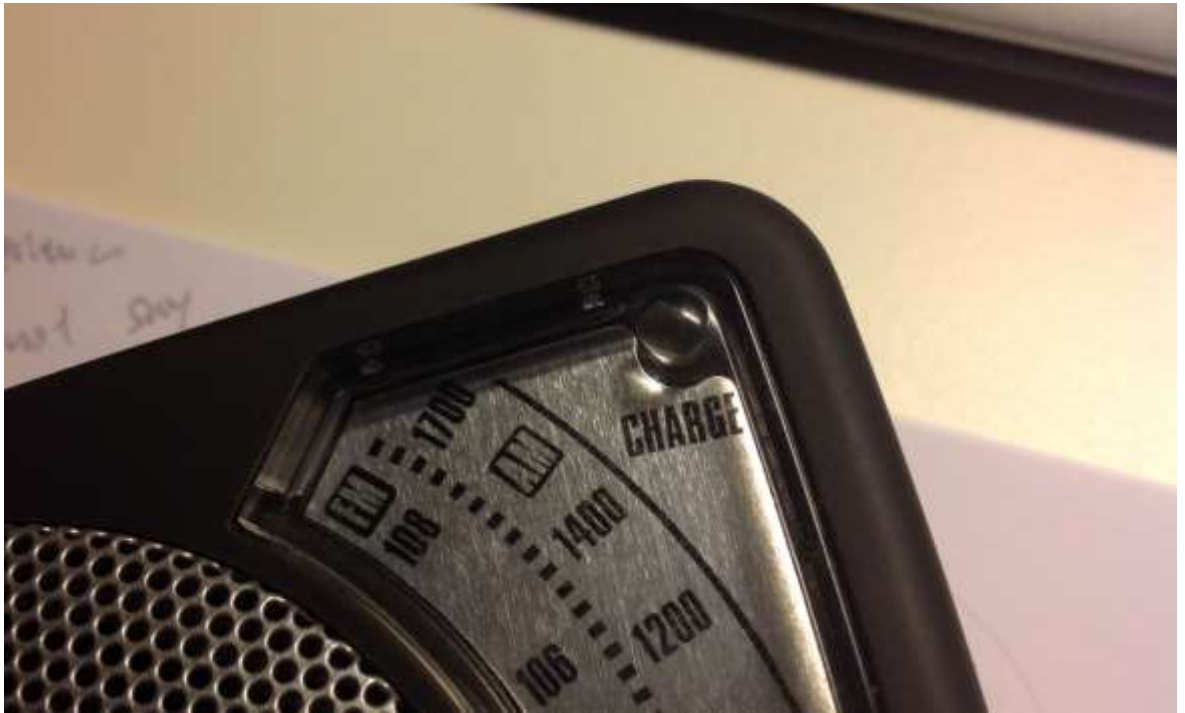
Figure 4.20 Charging indicator (LED) on HPP radio
