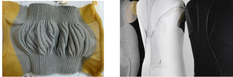
figure 1, left: knitted stretch sensor sample with steel yarn figure 2, right: three backs with integrated stretch sensor
