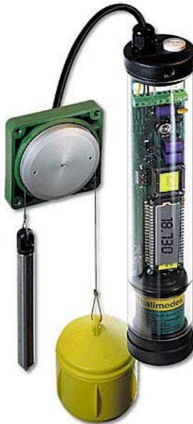
Using automated equipment, it is possible to monitor hydrological response on a very fine temporal scale. Typically this is at 5 or 15 minute intervals, although these figures can be adjusted depending on the required monitoring regime – more frequent monitoring increased data storage and therefore such units will require more frequent downloading. This resolution allows, for example, response to single rainfall events to be recorded very accurately.
